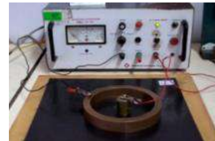
Electrical Resistance Test
