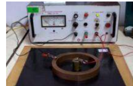
Electrical Resistance Test
